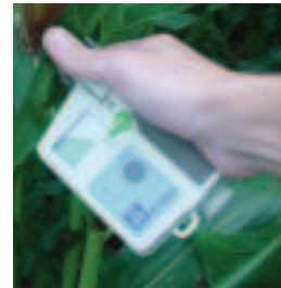
The N-Tester enables the farmer to read the nitrogen status of a crop from the green color of its leaves.
